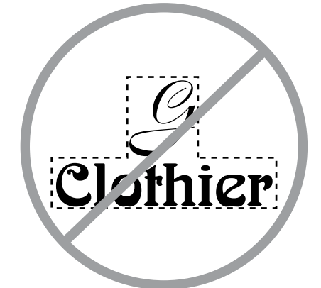
2. Improper method of tenant sign area calculation due to multiple geometric shapes
